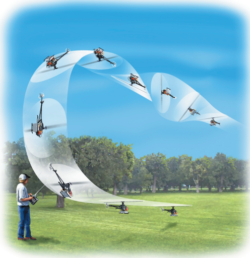
Figure 1: Miniature helicopter undergoing a Split-S maneuver. The same maneuver was performed by MIT helicopter under computer control. Drawing courtesy of Popular Mechanics magazine.
